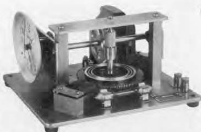
The TYPE 411 Synchronous Motor integrated applied frequencies to give an absolute evaluation in terms of standard time
