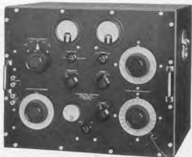
The second step, TYPE 600-A Standard-Signal Generator, for rapid measurements on broadcast receivers at selected frequencies, August, 1931
