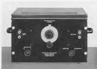
The TYPE 536 Distortion-Factor Meter measures the 400-cycle distortion in an audio-frequency system
