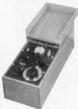
Ten thousand megohms on a bridge! — by means of the vacuum tube used in the TYPE 544 Megohm Meter
