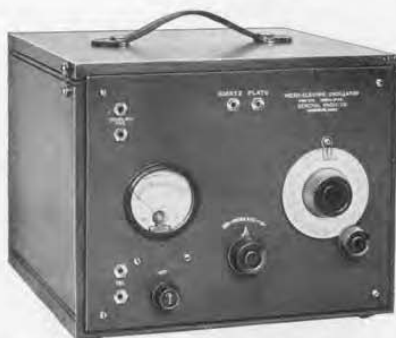
The early TYPE 275 Piezo-Electric Oscillator made no provision for temperature control of the Quartz Plate
