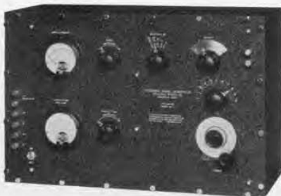
The first commercial Standard-Signal Generator, General Radio TYPE 403-A, November, 1928
