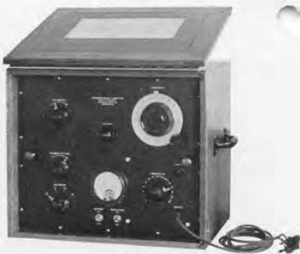
A simultaneous development for servicing and testing over a wide frequency range, the TYPE 601-A Standard-Signal Generator of July, 1931
