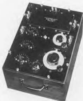
The TYPE 516-C Radio-Frequency Bridge measures impedances directly at frequencies up to 5 megacycles
