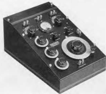
The refinement of decade bridges leads to specialized impedance bridges of greater usefulness in smaller fields, such as the TYPE 216 Capacity Bridge left , and the TYPE 650-A Impedance Bridge right
