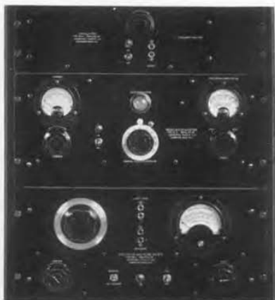
The CLASS 730-A Transmission Monitoring Assembly, introduced January, 1935, permits rapid routine measurement of modulation, distortion, and carrier noise
